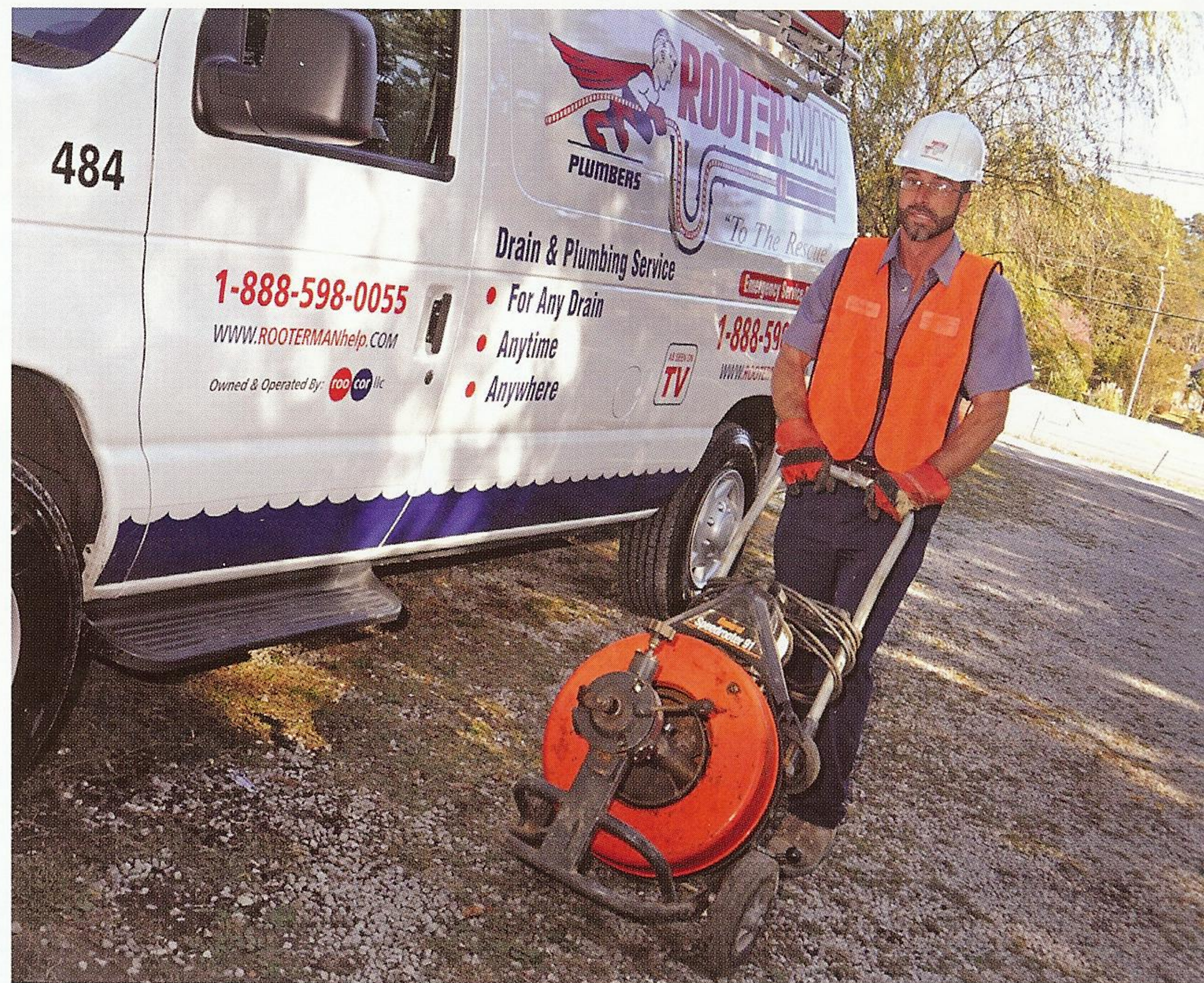
Service technician Loren Potter unloads a Speedroooter drain-cleaning machine from General Pipe Cleaners to take on a residential job.
